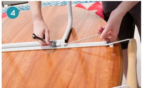
To tighten the screws we will need a wrench nº 13 and an Allen key nº 6.
